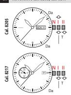
Time adjustment: Pull out the crown at position 2 and adjust the time by turning it counter-clockwise, then push the crown back into its neutral position [ N ]. Date adjustment: Pull out the crown till position 1 and adjust the date by turning it counter-clockwise, then push the crown back into its neutral position [ N ]. Weekday adjustment: Adjust the day by rotating the crown clockwise in 1 position.
